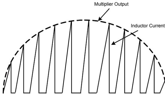
**Figure 4: Power-Factor Correction**
