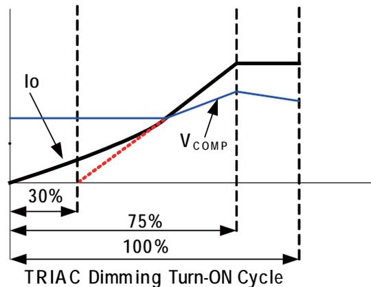
Figure 13: Dimming Curve
