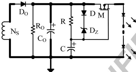
**Figure 14: Ripple Suppressor**
