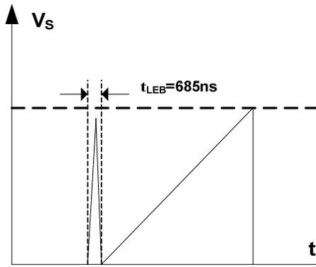
**Figure 7: Leading-Edge Blanking**
