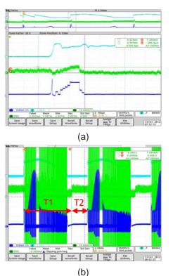
Fig. 4 Bleeding with Leading Edge Dimmer Ch1: Emitter current; Ch2 Vin sense; Ch4: Base current
