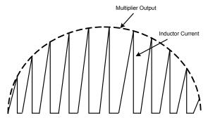
**Figure 4: Power-Factor Correction**
