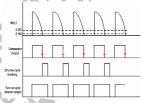
Figure 12: Dimming Turn-On Cycle Detector
