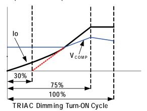
Figure 13: Dimming Curve
