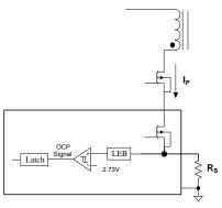
**Figure 10: Over-Current Protection Circuit**
