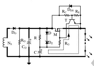
Figure 16: Drain-Source OVP and OCP Circuit
