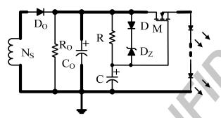
Figure14: Ripple Suppressor
