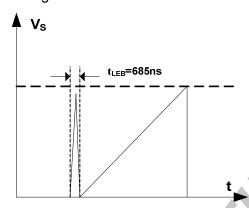
Figure 7: Leading-Edge Blanking
